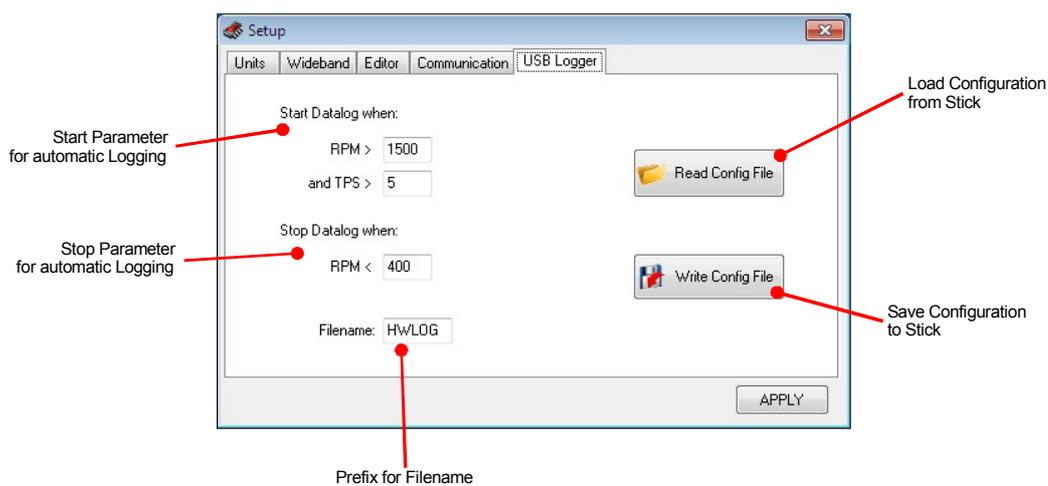
If you don't want automatic logging, just set the Start RPM value to 24000. The Filename can be only 5 chars long, because the Logger using the old 8+3 Filename System. The other 3 digits are filled by the Logger with a individual number for each file.
