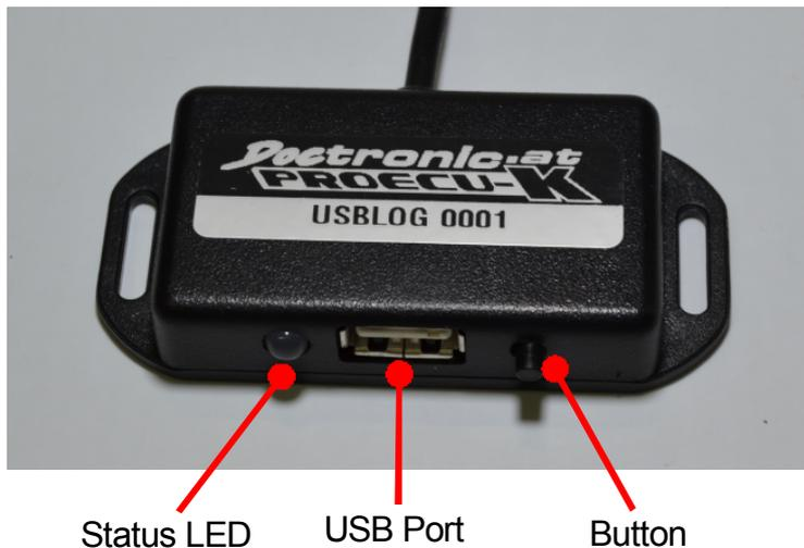
Beside of automatic start/stop of logging you can start and stop logging with the button. This is helpful when you want to remove the Stick while it is still logging.
