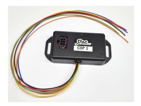
To install the COP2 Module you need to solder just 6 wires to the ECU board.
