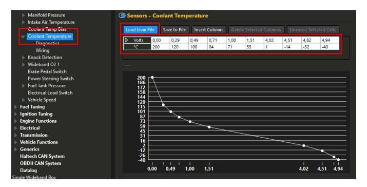
Enter Voltage to Temperature curve or Load from File. You can download our Coolant Temperature calibration from our website.
