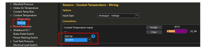
Disable the Pull Up Resistor for the Colland Temperature Input.
