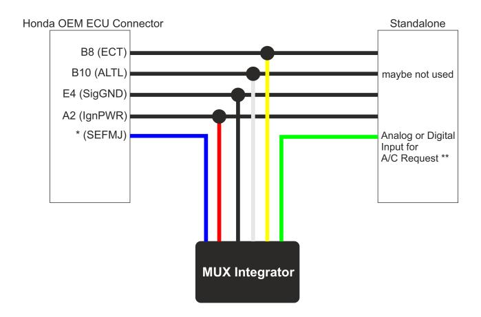
\* The Pin Location of the SEFMJ signal depends on the year and model of the ECU. Here a list of we know. For other ECUs refer the service manual for the pinout of the ECU.
