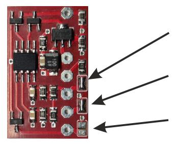
Enables a 4k7Ohm Pull-Up resistor to 12 Volt on the ALTL Line.
